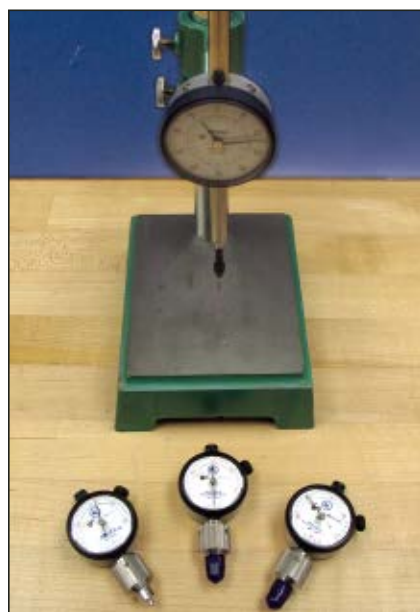
▲ Fig. 3 Gauges used to measure connector interfaces.
