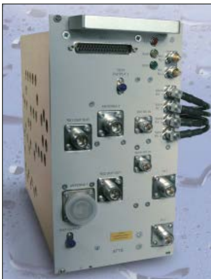
▲ Fig. 3 Application with high density connector population including waterproof QMAs on the right.
